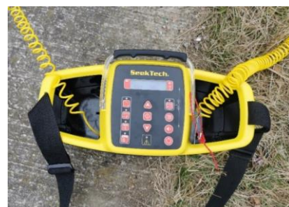
Fig. Error! No text of specified style in document..2 Ridgid SeekTech ST-510 line transmitter
