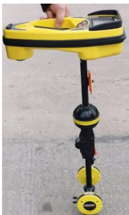
Fig. Error! No text of specified style in document..1 Ridgid SeekTech SR-60 Locator
