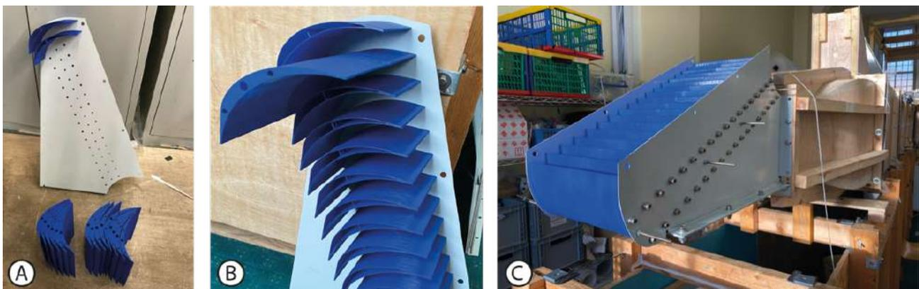
Fig. 11: Vanes being mounted to the side wall (A), a vane pair being joined (B), and the fully assembled vane cascade with bolted connections clearly visible (C).
