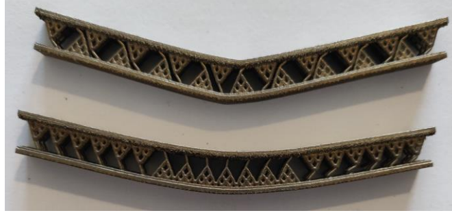
Figure 8. Sample SJ and S, after bending
