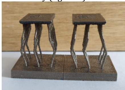
Figure 7. Samples S and SJ after compression
