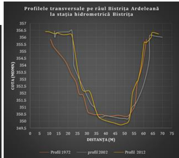
Figure 4.3 Transverse profiles of the riverbed at the Bistrița hydrometric station section.
