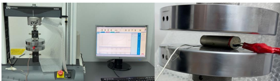
Figure 2. Uniaxial compression test of the battery performed on a universal testing machine.
